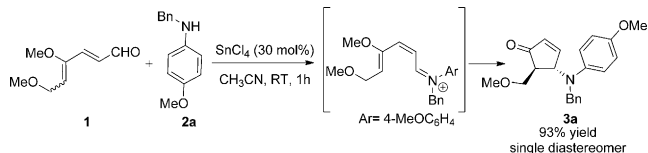
Scheme 2. Imino-Nazarov reaction of iminium ion generated from condensation of 1 and 2a .
